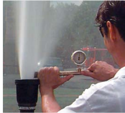
Testing exit pressure on a combination nozzle using a pitot tube. (Notice the smaller droplet size on this older style 100-psi nozzle)
