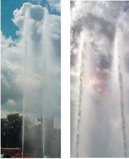
The first shows both streams side by side, while the second provides a closer view of the tops of the streams. Both streams are flowing equal gallons at equal inlet pressures. Which one is from the smooth-bore?
